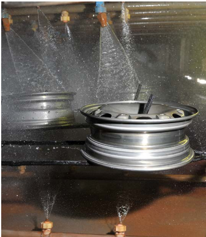
Cleaners may be used after machining operations (milling, cutting, drilling, grinding) to prepare the components for the next process stages such as assembly, adhesive-bonding, coating, painting or storage.
