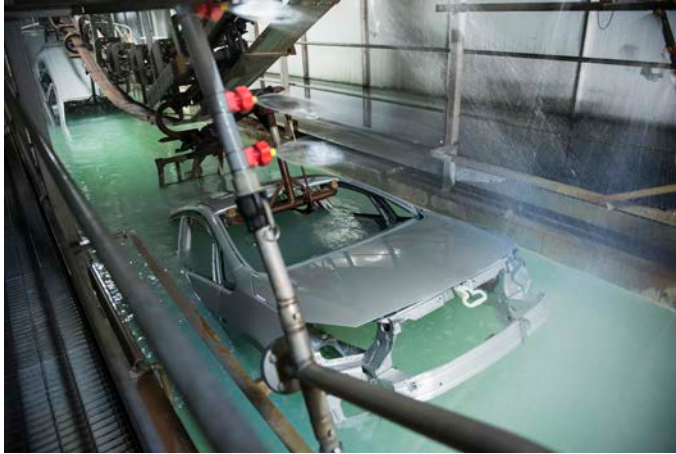
Dip baths used in the automobile industry ensure an even surface coating on the vehicle bodies.
