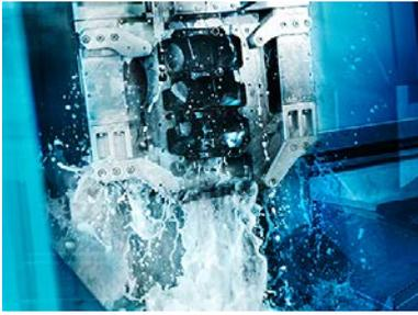
Cleaning high-quality and corrosion-resistant components such as engine blocks by using Bonderite C-NE 6250 in an industrial cleaning station exert a critical influence on final component quality.
