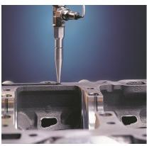
Henkel is able to offer polyacrylate-based cure-in-place liquid gasketing products which, thanks to their high flexibility and minimal permeability, ensure optimum results in the sealing of transmission control systems.
