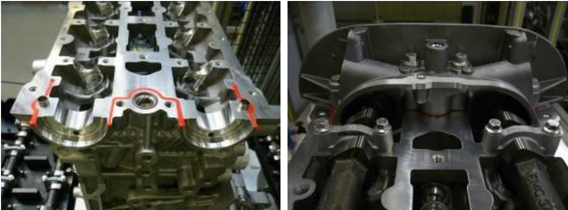
Highly stressed engine joints on Ford 1.0 and 1.6 liter EcoBoost engines are sealed with the anaerobic gasketing sealant from Henkel.
