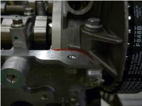
The “squeeze out” of the sealant at the interface with the cam cover and the rheology of the sealant ensures instant blow out resistance.
