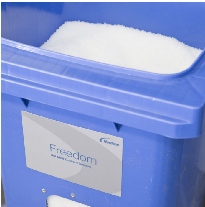
The hotmelt granulate is sucked from the feed box into the precision dispenser and only gets heated up to melt temperature just prior to application, considerably reducing the amount of energy consumed.
