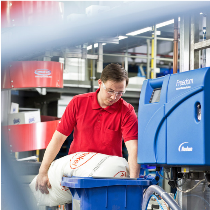
In the liquid laundry detergent production facility in Düsseldorf, Henkel employee Robert Hackl fills the blue hotmelt granulate feed boxes.
