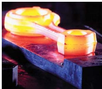
Forging lubricants are used in closed-die forging in order to ensure an optimal tool fill, controlled material flow and easy removal of the product from the die cavity.
