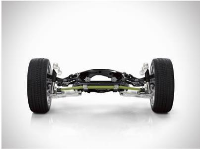
The rear axle of the new Volvo XC90 features a new transverse leaf spring, made of lightweight composite material. BENTELER-SGL mass-produces the composite leaf springs for the rear suspension using Loctite Matrix resin from Henkel.
