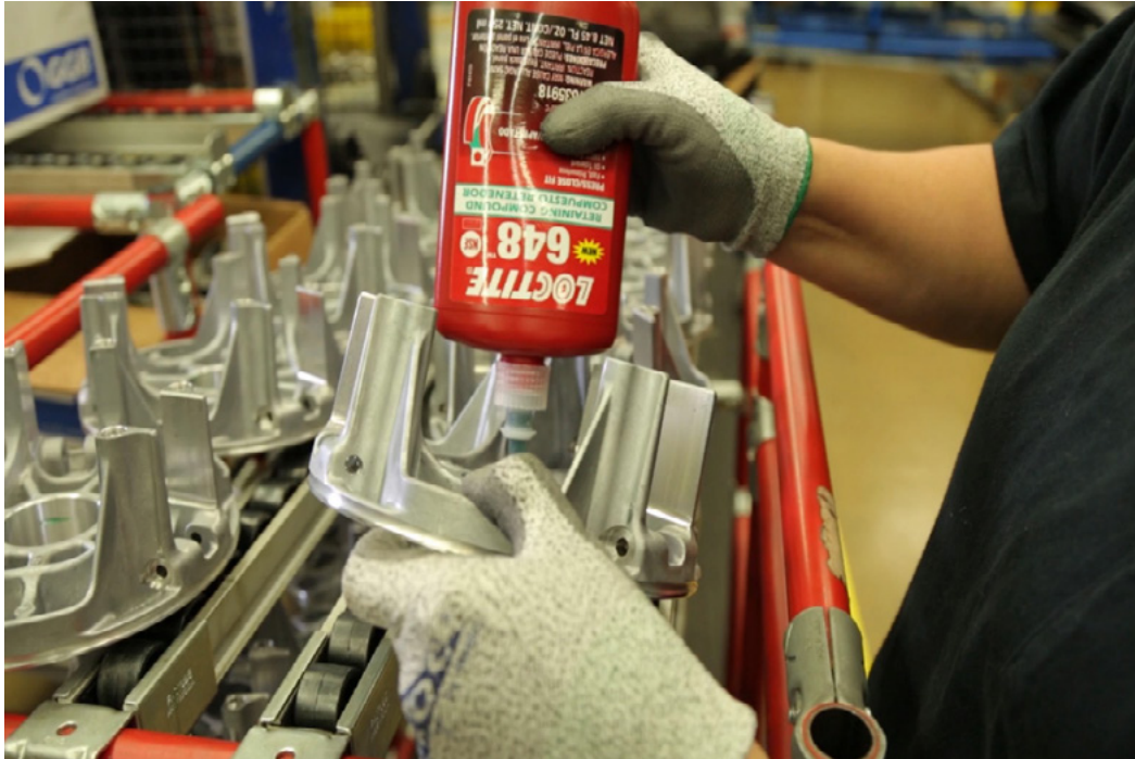
A Polaris operator applies LOCTITE 648 retaining compound to the inner diameter of the moveable sheave on the drive clutch assembly. Bearings will then be pressed into the part.
