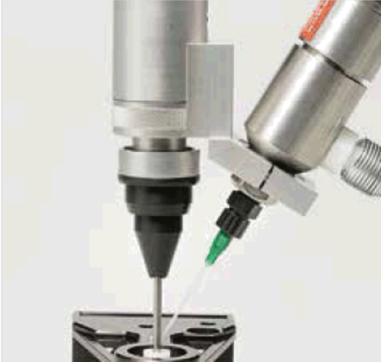
A specially engineered Rotospray applicator applies a metered amount of adhesive in a 360° bead or band onto a pre-defined location.
