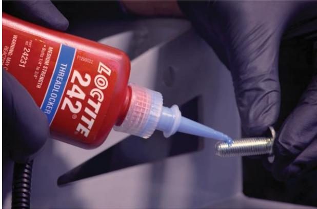
Threadlocker Loctite 242 makes sure nuts and bolts stay tight.
