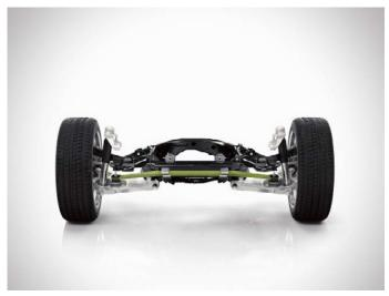
The rear axle of the new Volvo XC90 features a new transverse leaf spring, made of lightweight composite material. BENTELER-SGL mass-produces the composite leaf springs for the rear suspension using Loctite Matrix resin from Henkel. (Photo: Henkel, PR008)
