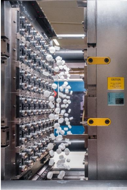
Ejection of screw caps for beverage bottles from a 96-mold tool with a 2.5 s cycle time at Corvaglia Closures Eschlikon (Image: Corvaglia)
