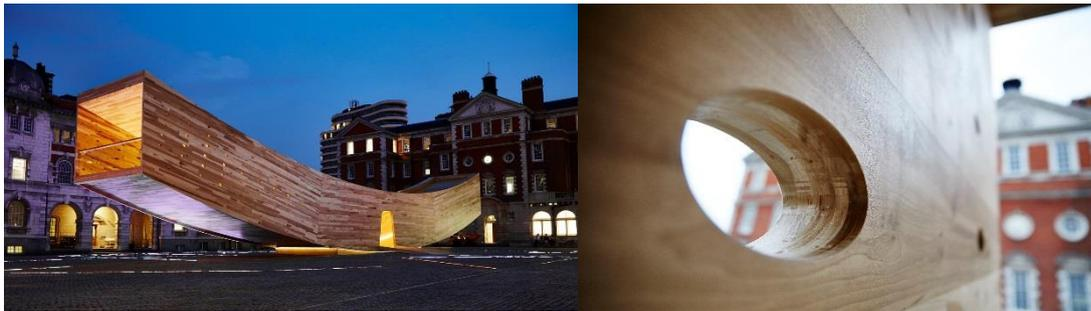
The curved form of the visitor-accessible, temporary art installation “The Smile” of cross-laminated tulip wood, which appeared at the London Design Festival, represents a smiling mouth. The components were bonded with an adhesive of the Loctite HB S Purbond line in combination with the newly developed primer Loctite PR 3105 Purbond. (Photos: Arup, [www.thetulipwoodsmile.info](http://www.thetulipwoodsmile.info))
