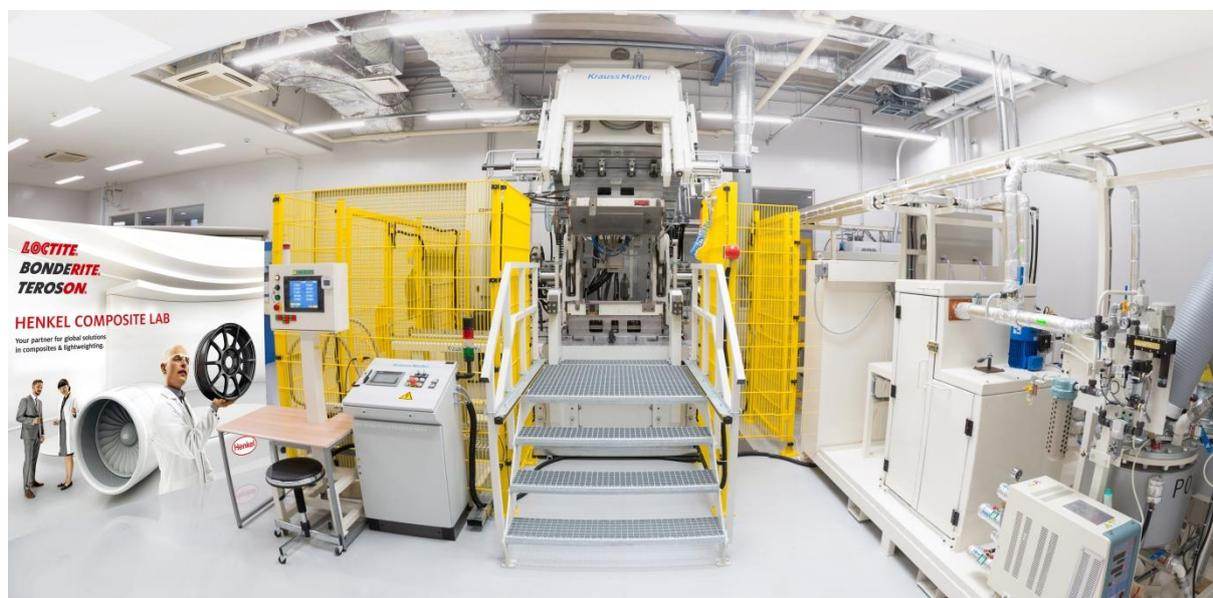
Henkel's new Composite Lab in Isogo-ku, Yokohama, Japan where automotive customers can work with Henkel experts to develop and test composite parts, and also optimize series production process conditions. They can carry out trials on Henkel's own HP-RTM equipment coupled to a 380-tonne press. (Photo: Henkel, PR035)
