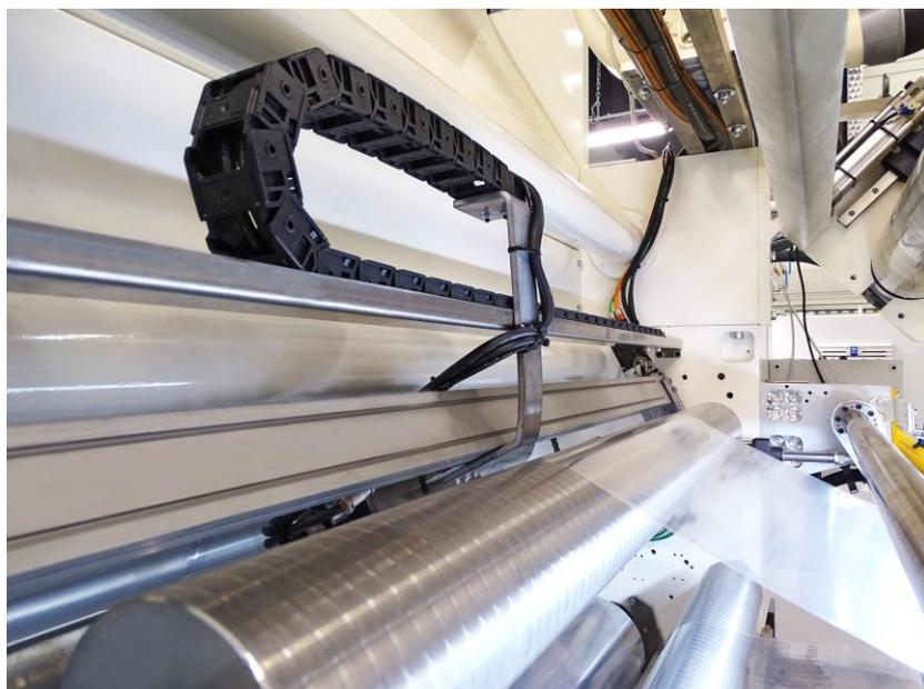
LiOSCAN is equipped with an oscillating infrared sensor moving along the film without contact to the material
