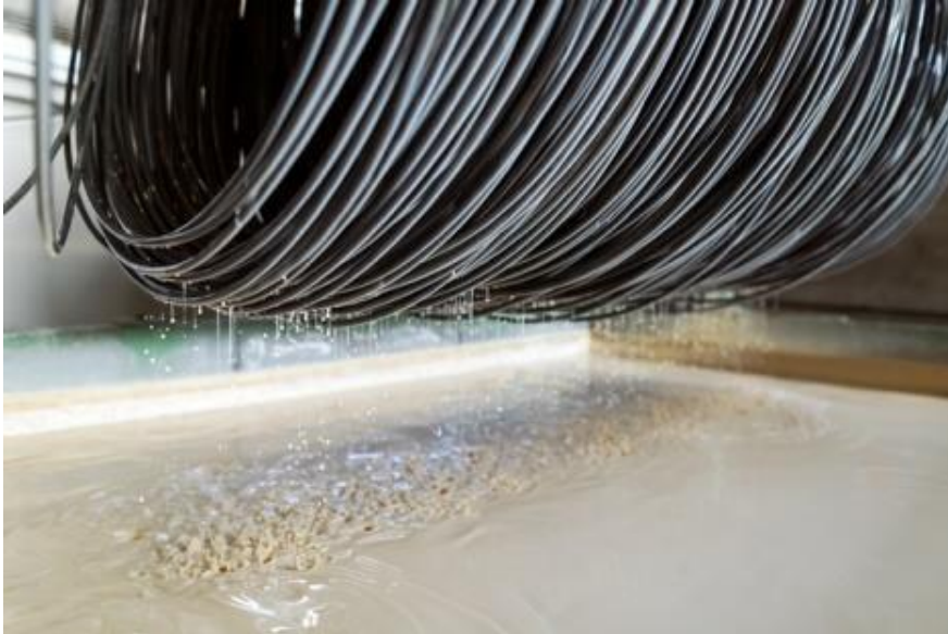
Bonderite L-FM FL is a water- based polymeric coating that enables a sustainable surface conversion process.
