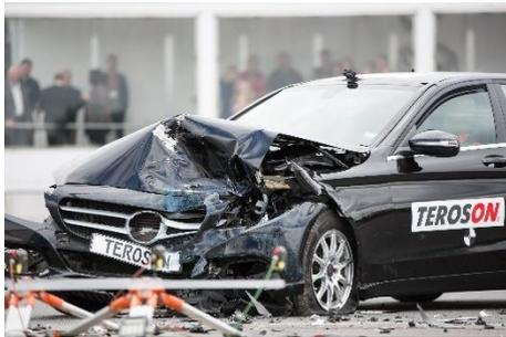
The results showed the windscreen bonded with Teroson adhesives, not only withstood the extreme crash test conditions, but also delivered the measured values required for the full functioning of the passenger airbag.
