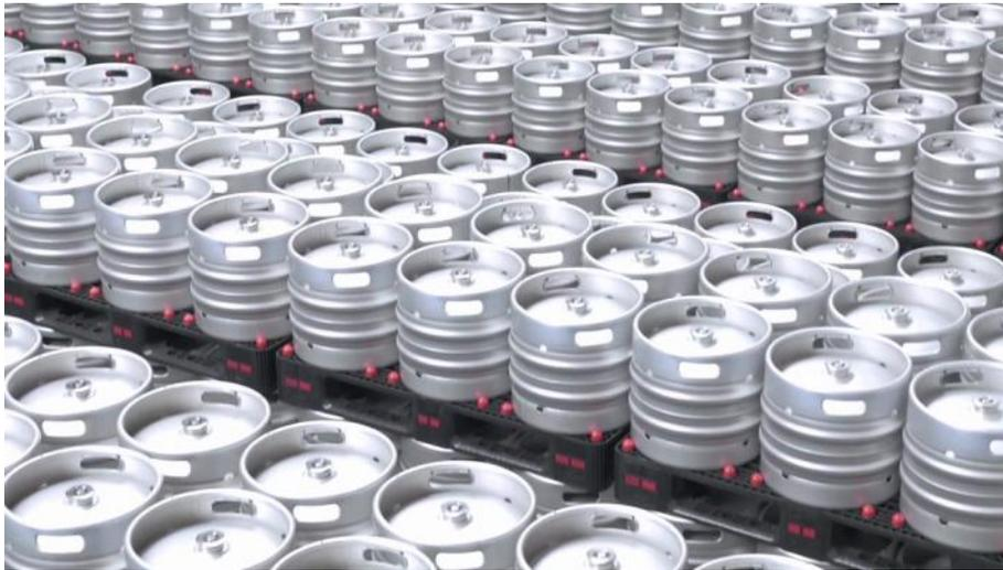
The new keg production plant of Entinox at Zaragoza, Spain, has a capacity for 450,000 barrels per year, made from austenite stainless steel with a surface of 2 square meters per barrel. (Photo: Entinox)
