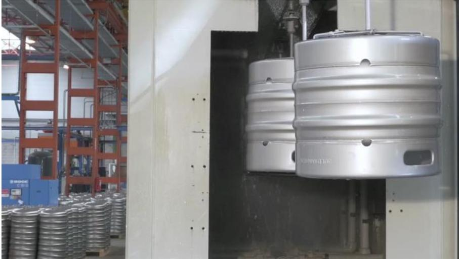
Kegs leaving tunnel after pickling with nitric acid-free Bonderite C-CP 1300. (Photo: Entinox)
