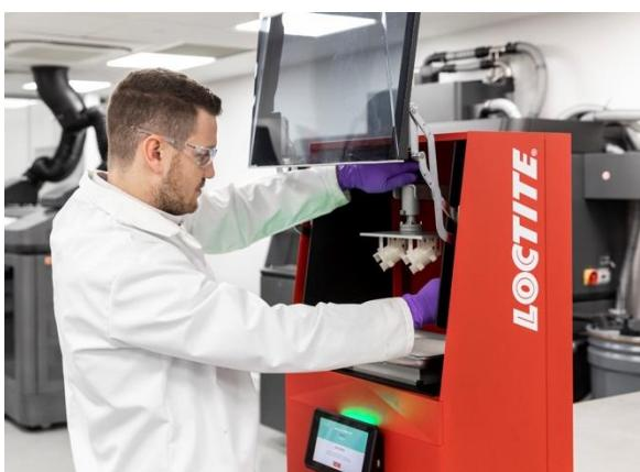
The Loctite 3D Printer is designed for professional use, including small series production and rapid prototyping.
