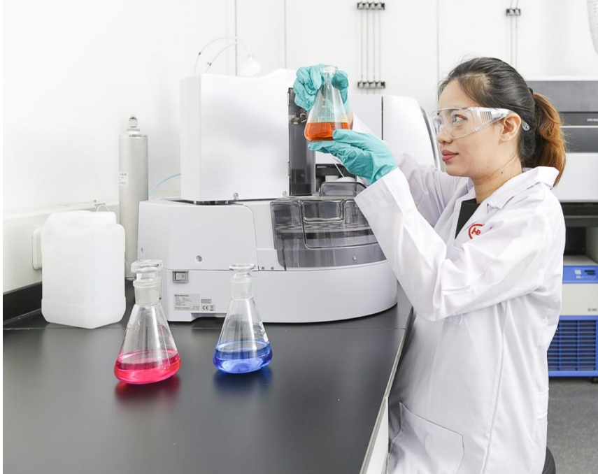
The total organic carbon tester is used to identify contaminants such as oil and bacteria in water or liquid solutions for the transport and metal industry.
