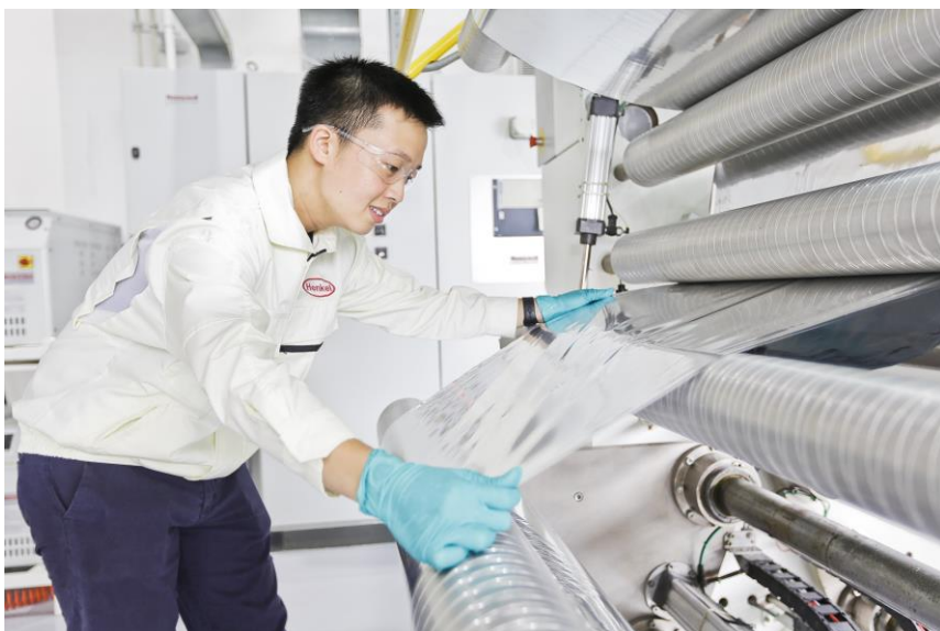
The state-of-the-art laminator machine is used to laminate flexible packaging for various products, such as food and shampoo sachets.
