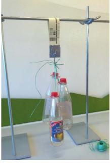
It might happen that the strips of paper will be damaged before the glue joint fails. This tells us that the glue is sufficient for its purpose – gluing paper.
